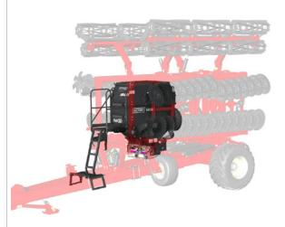
**Hydraulic** Two sets of hoses standard **Remotes** Additional hydraulic lines available
