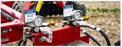
Down pressure on the HALO's hydraulically adjustable finishing systems is controlled by a valve on the tongue of the machine.
