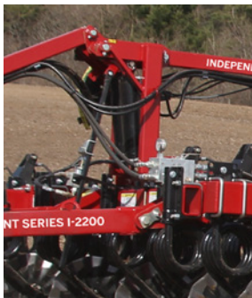
Salford Coil-Tech I models are equipped with a 4 bolt hub carrying a 20 inch blade. Salford Coil-Tech II models are equipped with a 5 bolt hub carrying a 22 inch blade.
